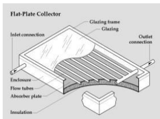
**Liquid flat-plate collector's** heat liquid as it flows through tubes in or adjacent to the absorber plate. The simplest liquid systems use potable household water, which is heated as it passes directly through the collector and then flows to the house. Solar pool heating this home in Nevada has an integral collector
