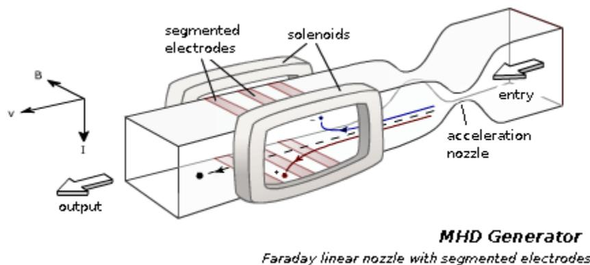
A magneto-hydrodynamic generator (MHD generator) is a magneto-hydrodynamic device that transforms thermal energy and kinetic energy into electricity. MHD generators are different from traditional electric generators in that they operate at high temperatures without moving parts. MHD was developed because the hot exhaust gas of an MHD generator can heat the boilers of a steam power
