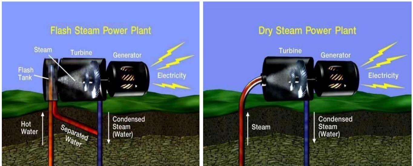
**Figure 2: Flash and Dry Steam Power Plant Diagrams**
