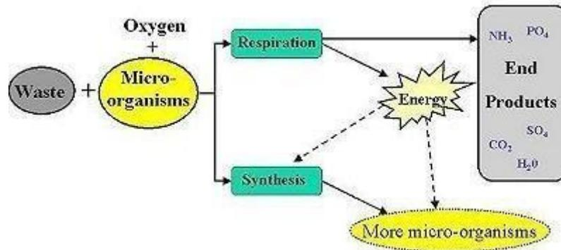
Path of Aerobic Digestion
