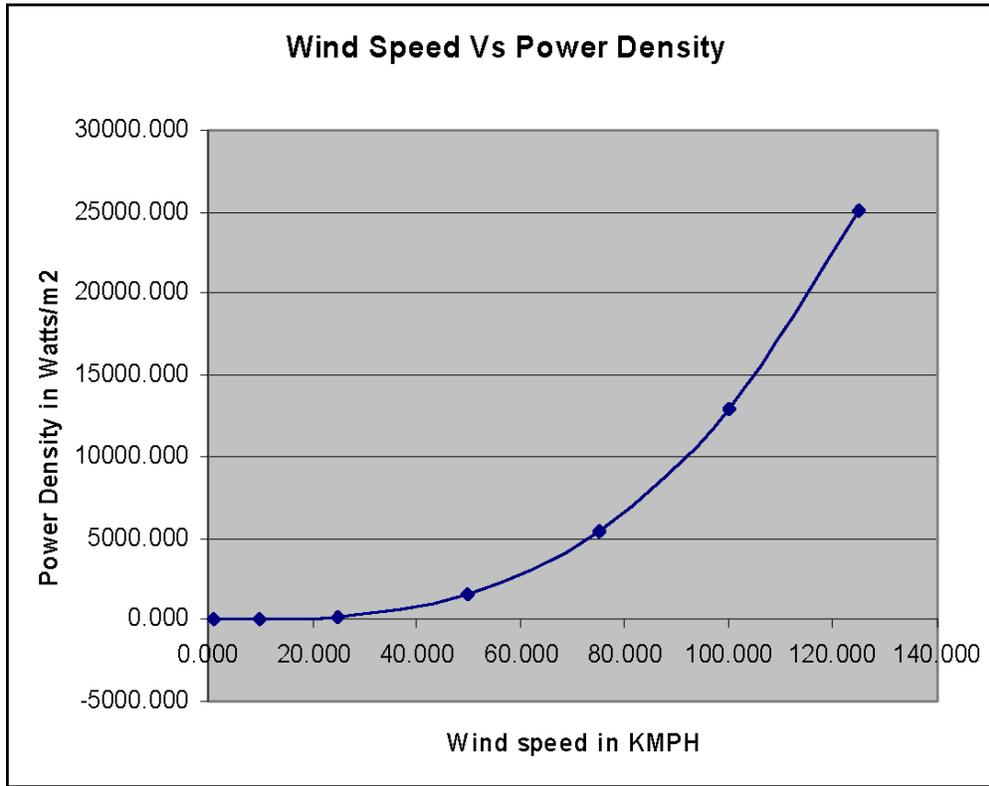
In the last column of the table, we have calculated the output of the turbine assuming that the efficiency of the turbine is 30%. However, we need to remember that the efficiency of the turbine is a function of wind speed. *It varies with wind speed.*
