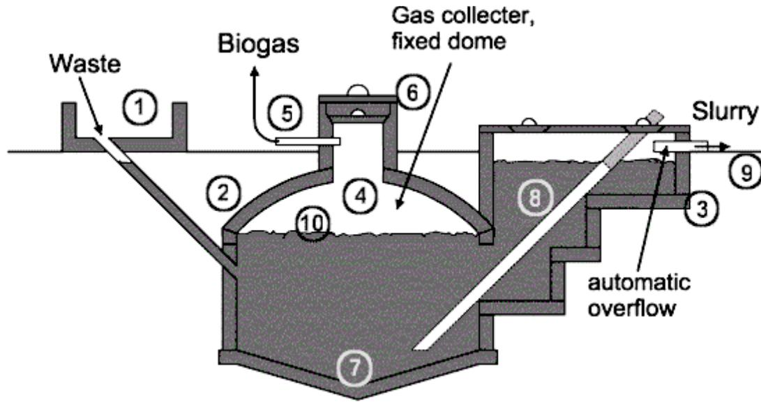
Figure 1: Fixed dome plant Nicaragua design: 1. Mixing tank with inlet pipe and sand trap. 2. Digester. 3. Compensation and removal tank. 4. Gasholder. 5. Gaspipe. 6. Entry hatch, with gastight seal. 7. Accumulation of thick sludge. 8. Outlet pipe. 9. Reference level. 10. Supernatant scum, broken up by varying level.
