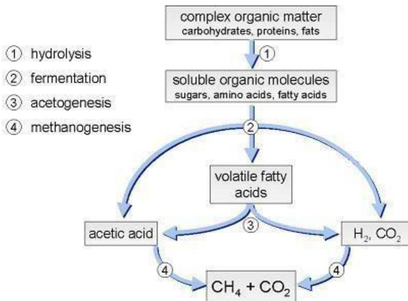
Path of Anaerobic Digestion
